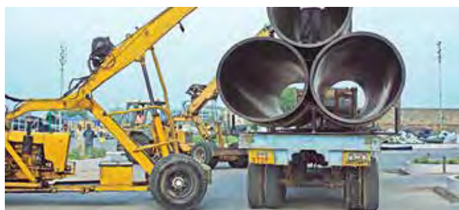
1600 mm PE Pipes used for safely conveying water over long distances (2009)
